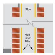
The flue can be lined with a heat resistant material such as clay or ceramic, and protects the structure of the chimney from both moisture and the heat of the rising gases from a fire.
