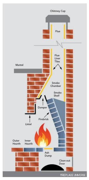
The diagram shows the layout of a fireplace and chimney commonly found in a home, but as all houses are built differently the layout and design of your fireplace may differ from the one shown above. For example, my open fireplaces don't have dampers or ash pits.
