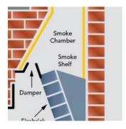
The smoke shelf also collects and helps to protect the firebox from any water or debris that makes its way down the chimney.
