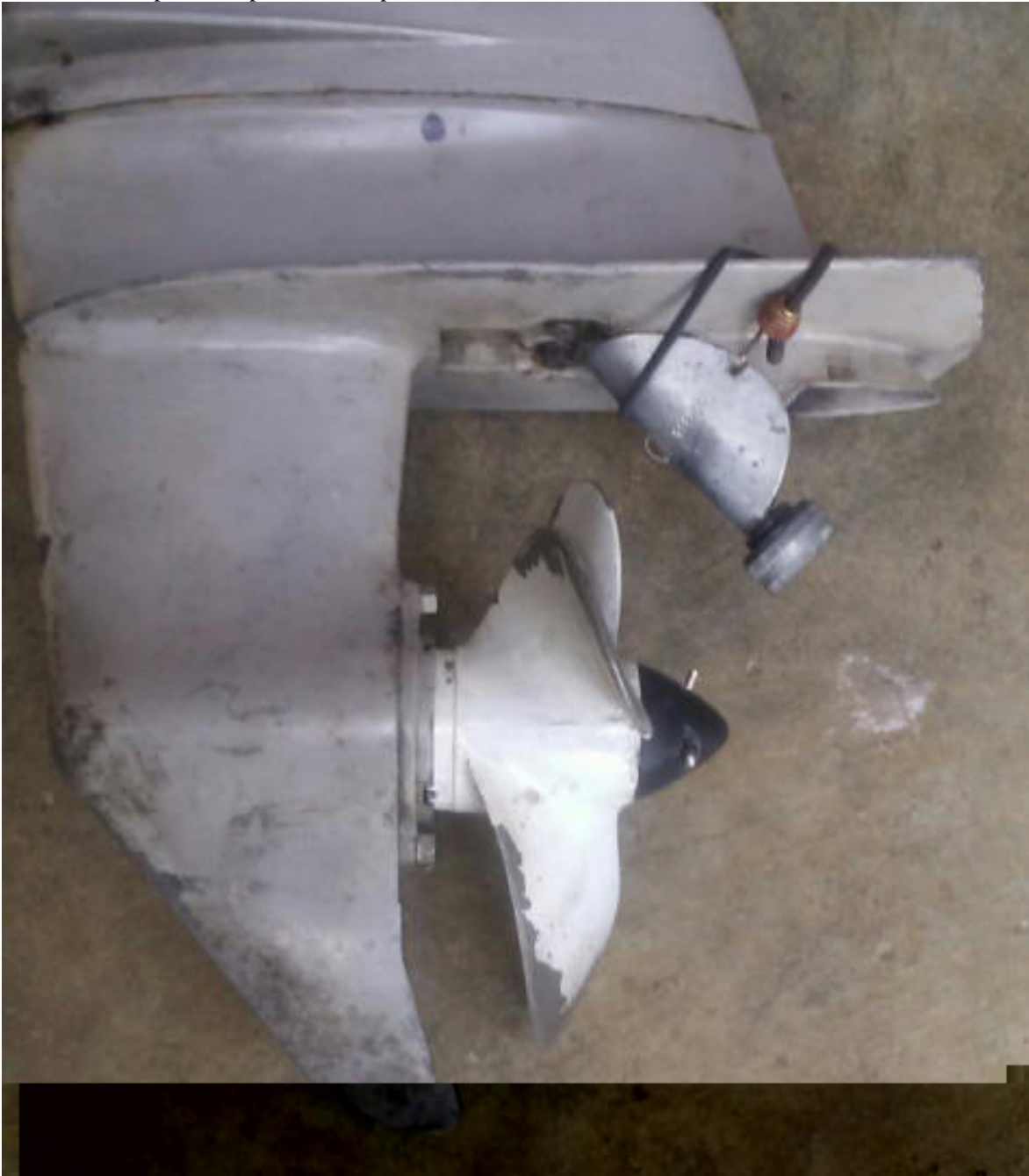
1984 Johnson 6hp with Tempo Flush Kit in place
