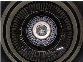
Front view of an A319-112 CFM56-5B6 with its fan removed
