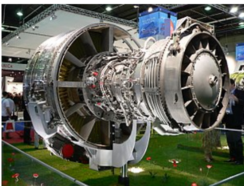
CFM56 Rear view of a CFM56-5 Type Turbofan National origin France/United States Manufacturer CFM International First run June 1974 Major applications Airbus A320 family Airbus A340-200/-300 Boeing 737 Classic / Next Gen Boeing KC-135R Stratotanker McDonnell Douglas DC-8-70 Number built 32,645 (June 2018)[1] Developed from General Electric F101 Developed into CFM International LEAP General Electric Affinity General Electric GE90
